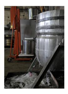
We create a physical process of molecular bonding activated by a low temperature heating of the monomer, about 50°C.
