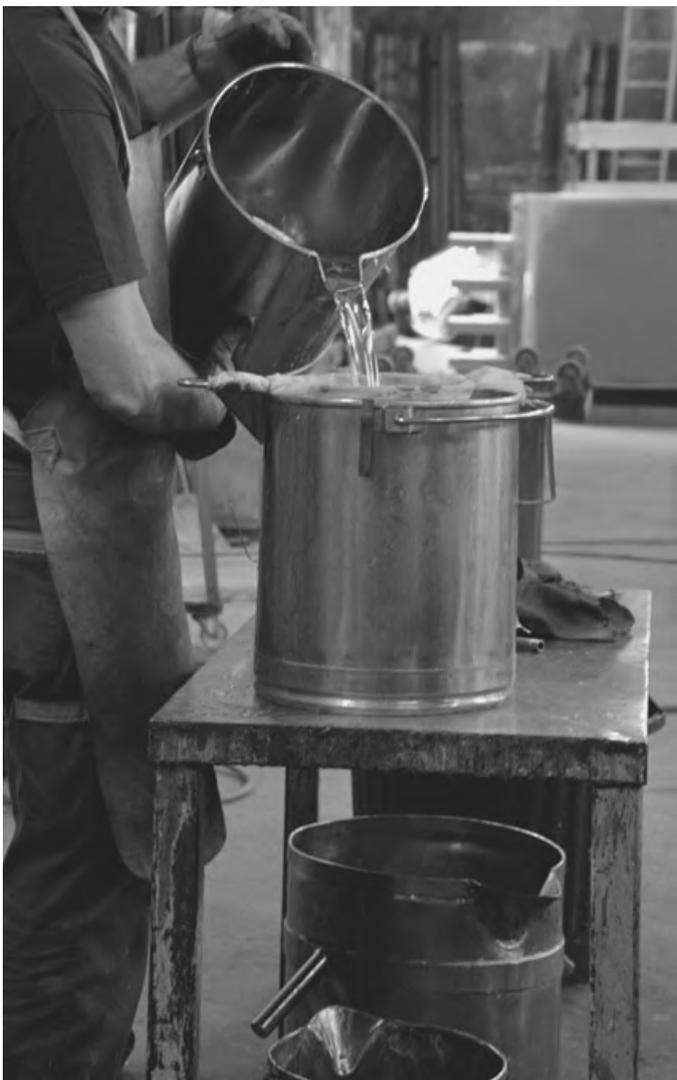
The polymerization of a Dacryl sheet is achieved by a physical principle of molecular bonding. This process is activated by heating the monomer at low temperature.
