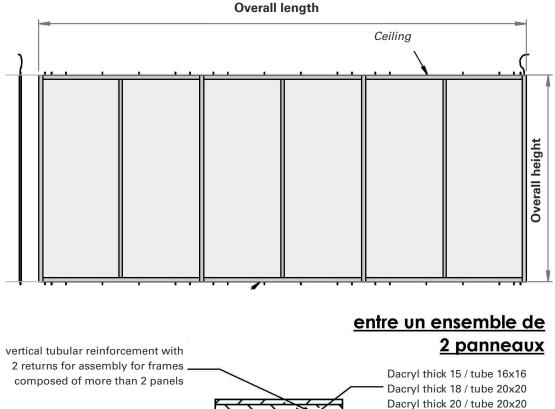
aluminium closing plates width 50 ep 4 removable with fasteners visible mechanics TFHC M3
